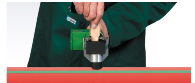
Heat-up of pipe ...
