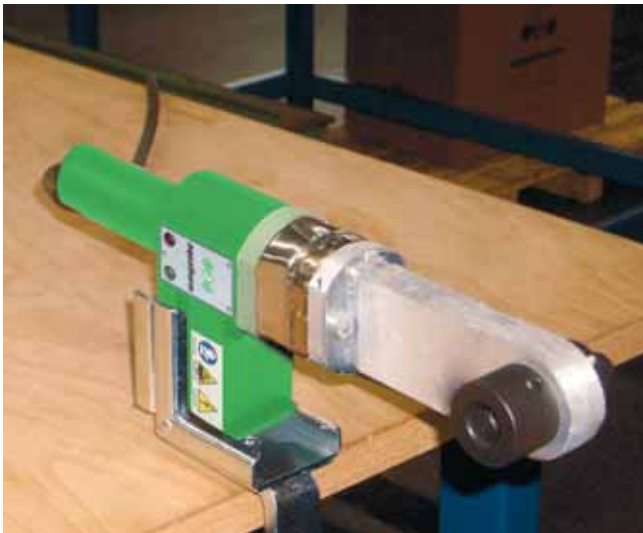
1. Mounted welding device and tools (16 mm) Control of temperature
